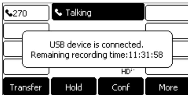
During a recording, if there is insufficient free space (30 minutes or 10 minutes left) on the USB flash drive, the IP phone will prompt you a message (XX minutes left for call recording). If no free space on the USB flash drive during recording, recording is stopped and saved in the USB flash drive automatically.
